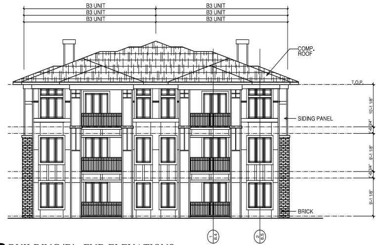
3 BUILDING 'D' - END ELEVATIONS SCALE: 1/8"=1'-0"
