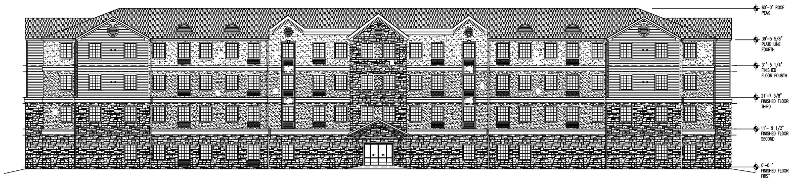
① FRONT BUILDING ELEVATION 3/32"=1'-0"
