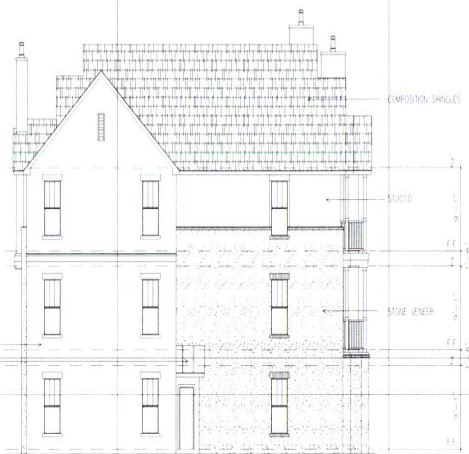
3 BUILDING 'A' END ELEVATION (BLDG. #6,11) SCALE 1/8"=1'-0"
