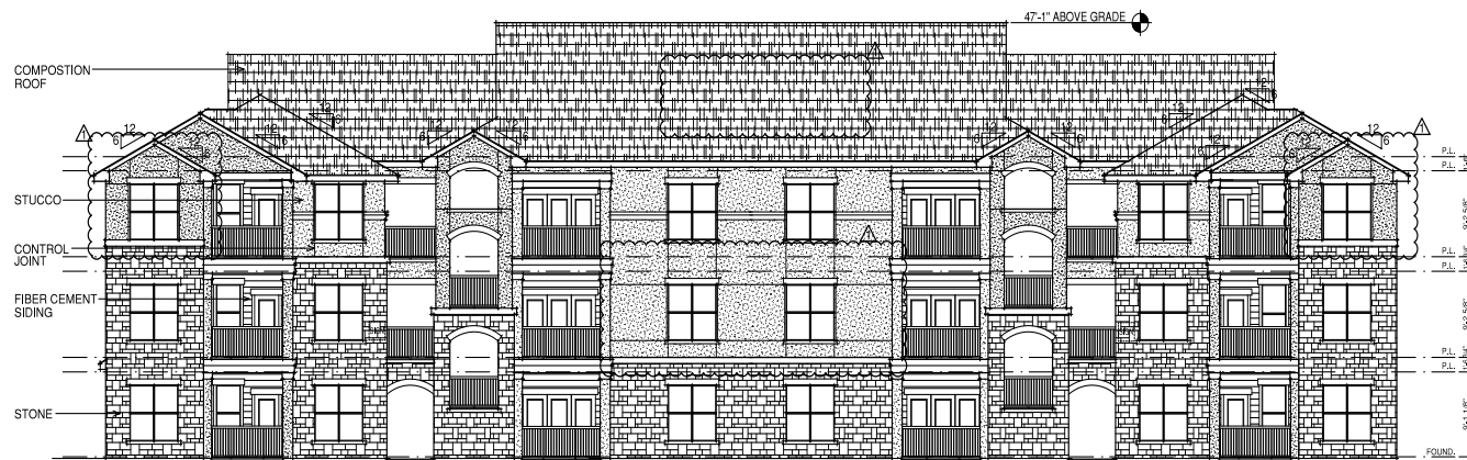
1 BUILDING 'E' FRONT ELEVATION - BUILDING(S) #12 SCALE 1/8"=1'-0"
