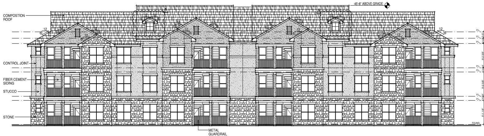
2 BUILDING 'A' REAR ELEVATION SCALE 1/8"=1'-0"
