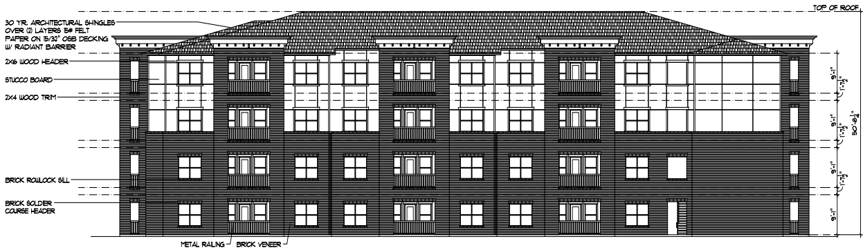
2 BUILDING ELEVATION - SOUTH 3/32" = 1'-0"
