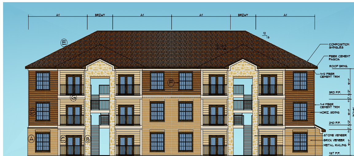
FRONT ELEVATION - BLDG. TYPE I
