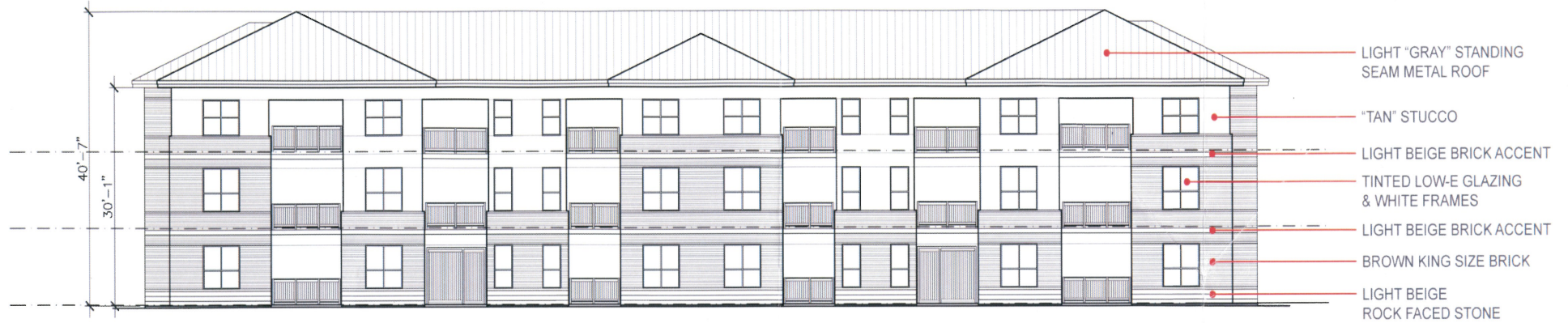
FRONT ELEVATION BUILDING A+B
