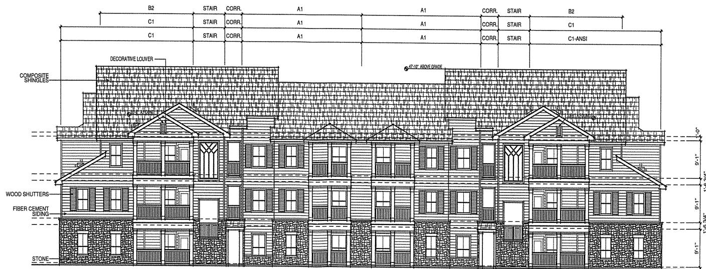
1 BUILDING 'C' FRONT ELEVATION (SIM COND. FOR BACK ELEV.) SCALE 1/8"=1'-0"
